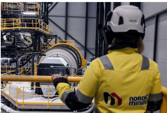
Figure 20 - Processing plant including crushing, grinding and separation of rutile and garnet concentrates. (Photo: Jostein Vedvik)
